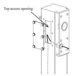
Figure 6 Connecting Wiring Through Pole
